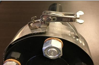
Step 3: Pull back the latch and tighten it by turning the wing nut clockwise until fully secured and locked.
