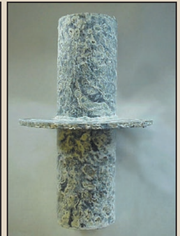
Figure 4: Galvanized Wall Sleeve after 500 hours of exposure
